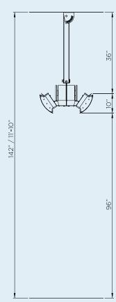
CEILING POLE CLEARANCE WITH HEAT DEFLECTOR
