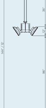
CEILING POLE CLEARANCE WITH HEAT DEFLECTOR
